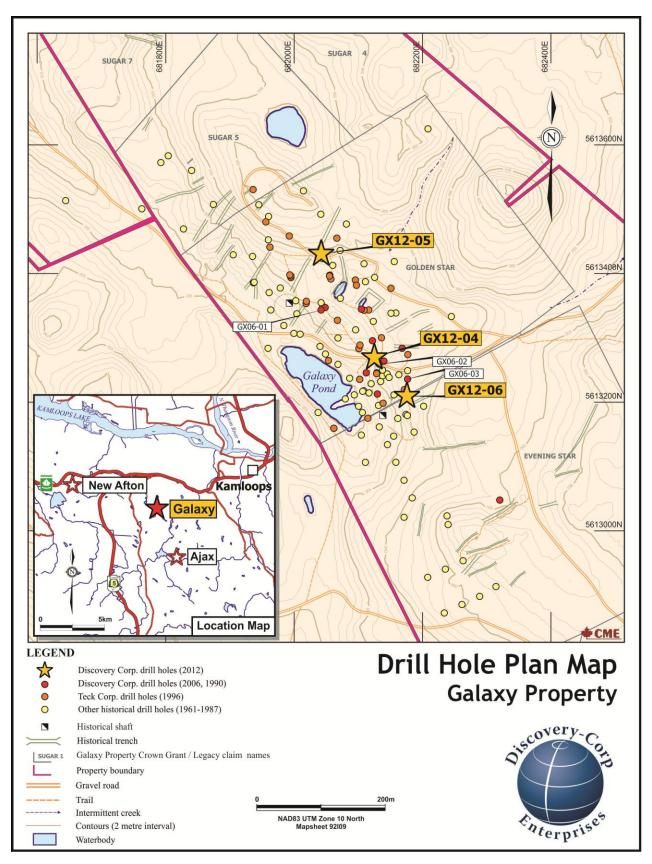
This Drill Hole Plan Map illustrates diamond drill holes GX12-04, GX12-05 and GX12-06.
